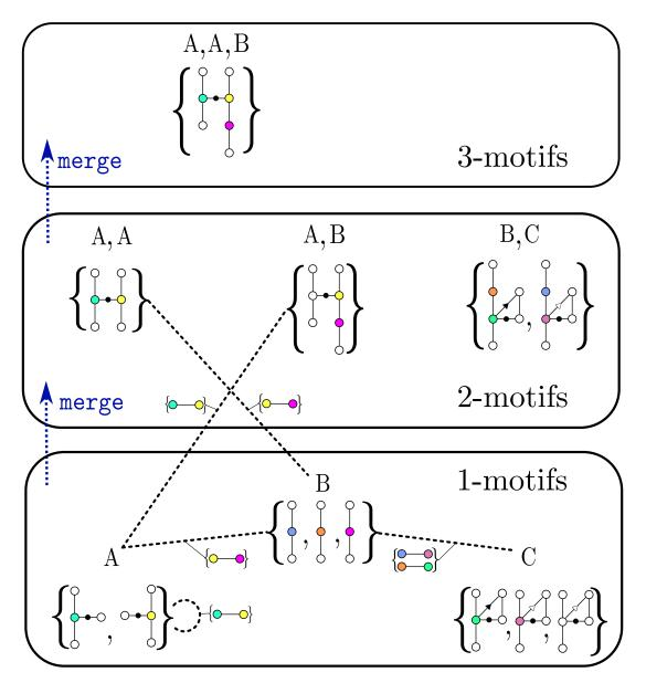
**Figure 4.2** – MAA Illustration : Meta-nodes A,B and C get merged into three 2-Meta-nodes AA, AB and BC. Then new meta-edges are computed that link singletons A and B with 2-meta-nodes AB and AA respectively. A second merge follows these links and yields the 3-meta-node AAB. Node colors here are a proxy for node ID, and not tied to the cluster IDs (A, B, C).
