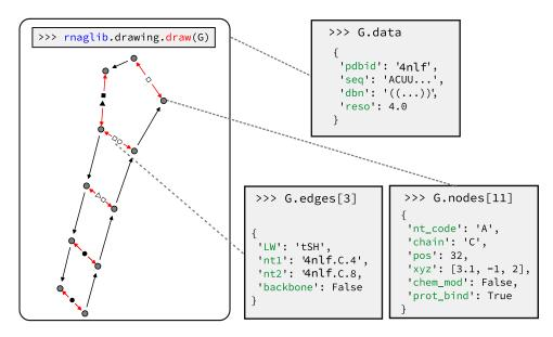
Figure 5.1 – 2.5D graph representation of the 23S ribosomal RNA Sarcin Ricin Loop (PDBID: 4NLF). Left panel shows the output of the drawing tool with default settings. Grey boxes are added later to depict a few of the attributes of the graph object, its nodes and its edges.
