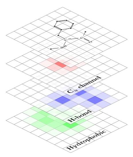
**Supplementary Figure E.1** – Visual representation of the grid embedding process. The different atom-types are encoded with a Gaussian density around the atom center in atom-types grids. Then these grids are stacked on top of one another.
