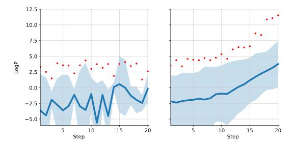
**Figure 8.4** – Composite logP optimization results : the blue curve plots the mean and standard deviation of the clogP at each iteration and the red dots show the maximum score. *Left:* Bayesian Optimization of clogP with 10k initial samples and 500 new samples per step, using implementation from Kusner et al. [2017]. *Right:* CbAS for clogP optimization, with 1k samples per step.
