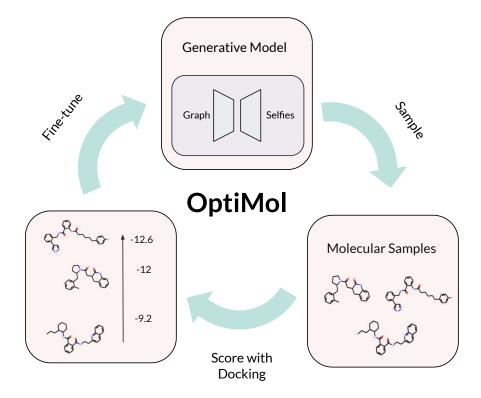
Figure 8.2 – OptiMol workflow: A prior generative model is trained on a broad chemical space and generates samples. We use docking to score these samples, and fine-tune the generative model on the samples weighted by their docking scores
