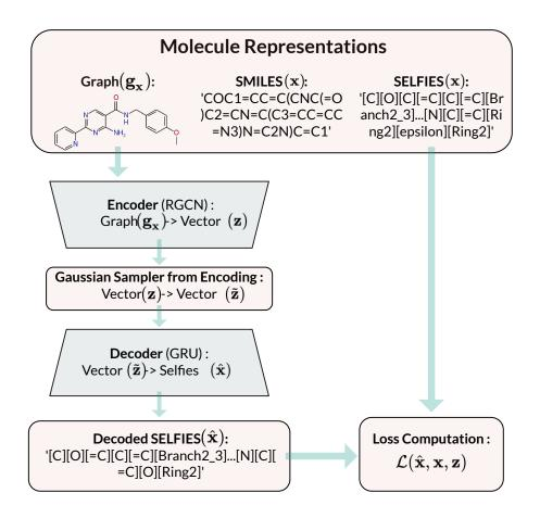
**Supplementary Figure F.1** – Training of the VAE : The molecule gets encoded based on its molecular graph into a vector through an Relational Graph Convolution Network. Then this vector gets decoded into a selfie using a Gated Recurrent Unit Network. Finally a loss gets computed between the decoded SELFIES and the canonical one representing the input molecule. The error is back-propagated through the network.
